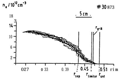
fig. 5 momentary profiles from 35 sweeps in a stationary plasma phase, superimposed (same plasma phase as in fig. 6,  $R=167.7\text{ cm}$ ) (  $B=2.8T, I_p=420kA, n_e=1.3 \times 10^{13}/cm^3$  )
