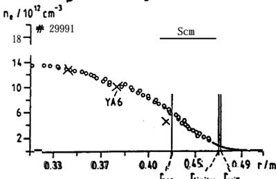
fig. 8 Comparison of the density profile measured with the reflectometer to the densities obtained with outermost channels of the Thomson scattering system (YAG). (  $B=2.8T, I_p=320kA, n_e=2.0 \times 10^{13}/cm^3$  )
