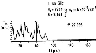
fig. 2 Intensity of the reflected signal from the plasma, fixed frequency; The launched signal has been chopped, so that the right part of the trace gives the baseline.
